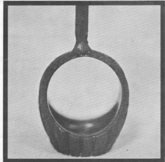
SPRUE ATTACHED TO WAX PATTERN SHOWING SMOOTH WELD
